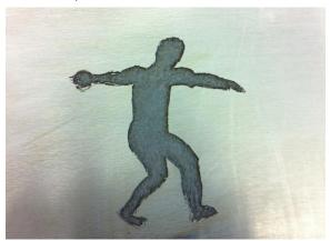
the bath. The tin ions then get reduced and precipitate out of the solution as tin metal
