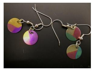
Niobium can also be oxidized to create art. The metal can be anodized in electrolyte solution at different voltages. At each different voltage a different thickness of oxidation forms and each different thickness appears to be a different color (below).
